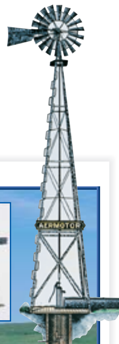
STEEL WINDMILL In regions of unpredictable rainfall, the steel windmill prevented crop dehydration by bringing up underground water for irrigation.
